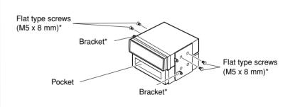
Note: When installing the receiver on the mounting bracket, make sure to use the 8 mm-long screws. If longer screws are used, they could damage the receiver.
